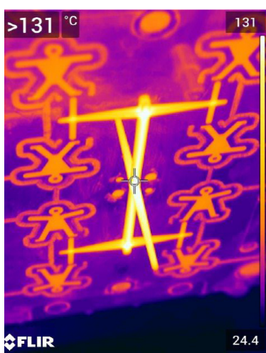
A. Experimental IR image after mold opening
