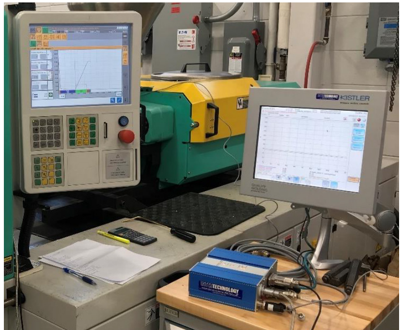
Fig. 6: Control and monitoring system, measuring sensor temperatures and mold conditions
